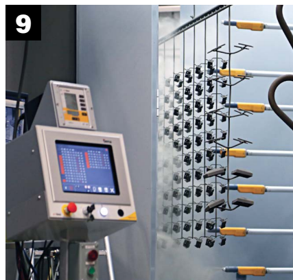
9 Powder is applied with 18 automated and 2 manual spray guns. Compressed process air is dried to -35°F Dew Point for superior adhesion.
