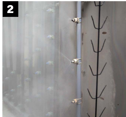
2 The product enters a heated cleaning stage to remove extrusion debris and fabrication oils.
