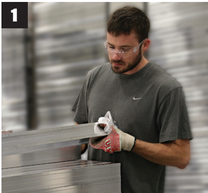
1 The raw premium-grade aluminum is inspected to be free of blemishes and is not exposed to the outdoor elements.
